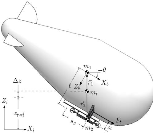
Fig. 1. Reconfigurable blimp model and coordinate system
