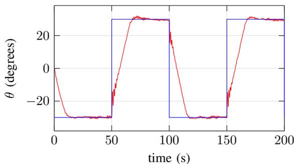
Fig. 5. Vehicle pitch angle (red) and reference pitch angle (blue) for square control signal
