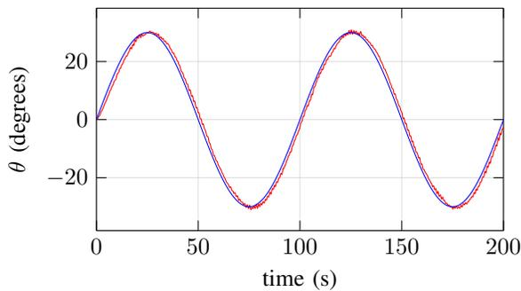
Fig. 4. Vehicle pitch angle (red) and reference pitch angle (blue) for sine control signal
