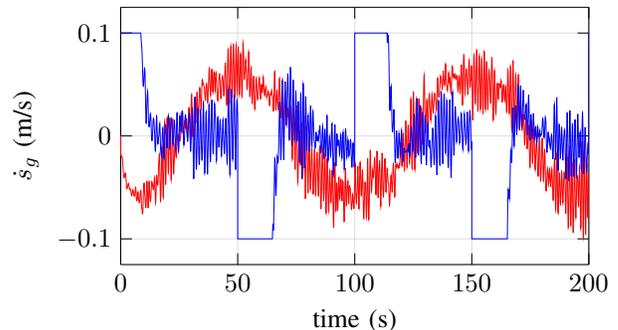
Fig. 9. Gondola velocity  $\dot{s}_g$  for sine (red) and square (blue) control signals
