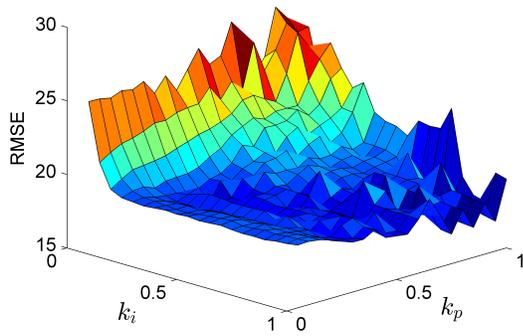
Fig. 3. Root mean square error of the pitch tracking for a step reference pitch trajectory with  $F_t = 3$  N and  $V_{\text{wind}} = 0.35$  m/s. Similar trends were observed at lower thrust levels and higher wind speeds.
