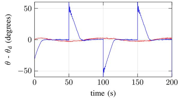
Fig. 6. Tracking error for sine (red) and square (blue) control signals
