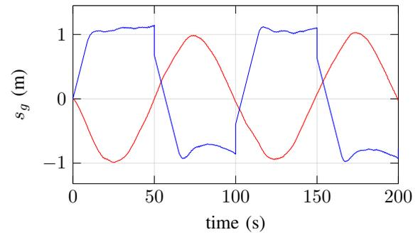
Fig. 7. Gondola position  $s_g$  for sine (red) and square (blue) control signals
